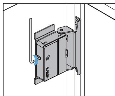
Closing speed of doors is adjustable with a hex key (size: 2.5).
