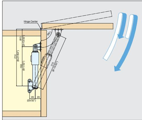
\*Lid stay must be installed parallel to the sidewall.
