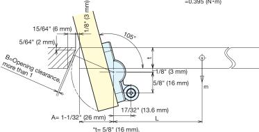
Installation Cross-section Drawing
